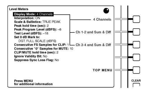
Figure 18: The Level Meters submenu
